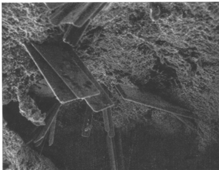
Fig. 3: Scanning electron microscopy photograph of hydrated cobalt molybdate compacts heated to 680^\circ and cooled at 25^\circ ( \times 800 )
